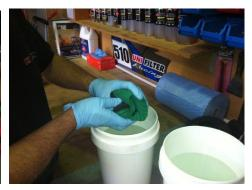
Step 3. Rinse foam in clean bucket of water to remove the dirt. If the filter is still dirty repeat this step.
