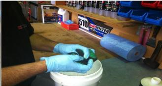
**Step 7.** Wrap the filter tightly in an absorbent towel or cloth for 20 mins to draw any excess oil out of the filter.
